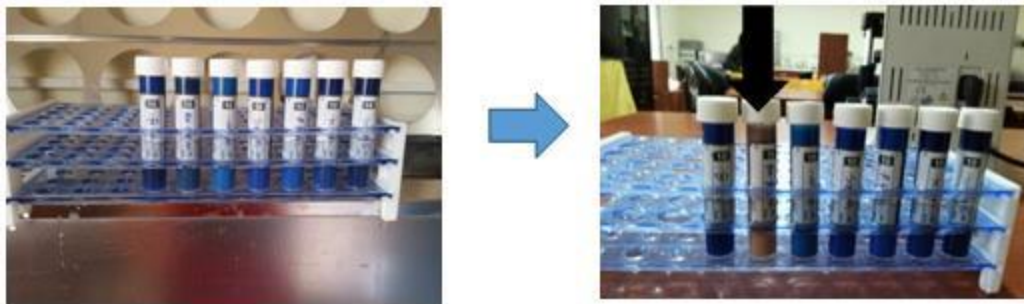
Fig.3.4: Different milk samples with different additives before and after addition of MB.
